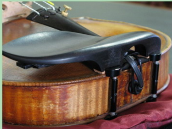
Chinrest mounted on the violin with the sensor inside the body
